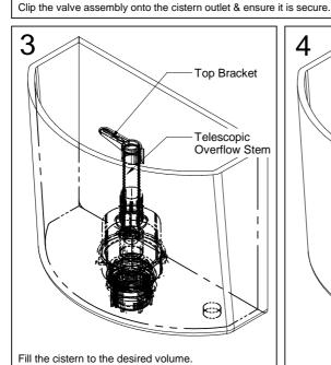
Adjust the telescopic overflow stem by turning it clockwise to loosen. Move the overflow stem up or down until the underside of the top bracket touches the water
