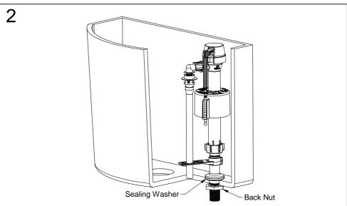
Insert valve into cistern with sealing washer on the inside of the cistern. **Do not use putty.** Position the valve, ensure the float is not in contact with the cistern & is able to move freely.
