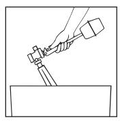
1. Turn off water supply to toilet cistern. Flush cistern and drain water.
