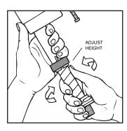
3. To adjust valve height, remove it from cistern. Twist threaded shank in or out of valve body without moving grey ring (height adjusts from 225mm. to 350mm. – the clicking noise heard is normal).
