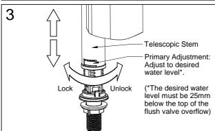
Adjust the valve height by turning the telescopic stem anti-clockwise to unlock.
