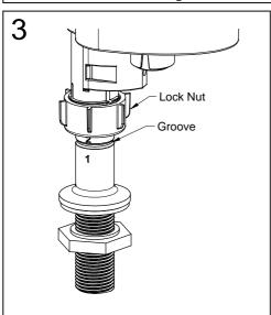
Adjust the valve height by loosening the locknut & moving the valve up or down to the desired height. The top of the valve should not protrude above the cistern rim.
