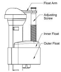
The desired water level can be adjusted by firmly moving the outer float up or down to achieve the required level and the inner float can be adjusted by screwing the adjusting rod in or out.
