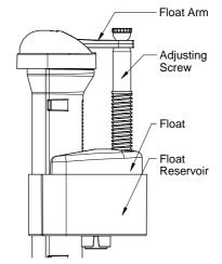
The desired water level can be adjusted by firmly moving the float reservoir up or down to achieve the required level and the float can be adjusted by screwing the adjusting rod in or out.
