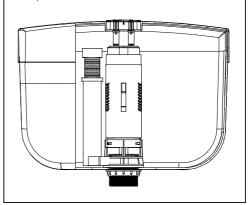
Button assembly: Fit the button assembly and the cistern lid to the cistern.
